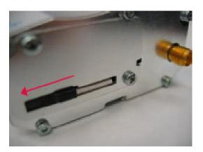
Use a tool to further push the SIM card into the SIM holder. Push until you hear a clicking sound.
