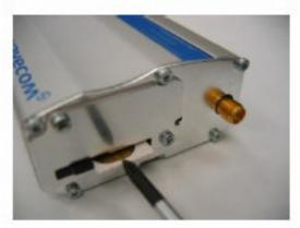
Slide the SIM lock switch to lock the SIM card in the Fastrack Xtend.
