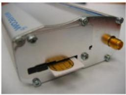
Use a tool to help push the SIM card into the SIM holder. Push the SIM card all the way in until you hear a clicking sound.
