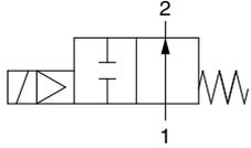
When the valve is closed, flow is blocked from port 1 to port 2. However, if the pressure in port 2 is higher than port 1, the valve will not be able to block the fluid and it will flow from port 2 to port 1.
