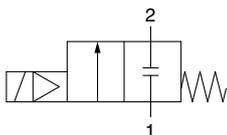
When the valve is closed, flow is blocked from port 1 to port 2. However, if the pressure in port 2 is higher than port 1, the valve will not be able to block the fluid and it will flow from port 2 to port 1.
