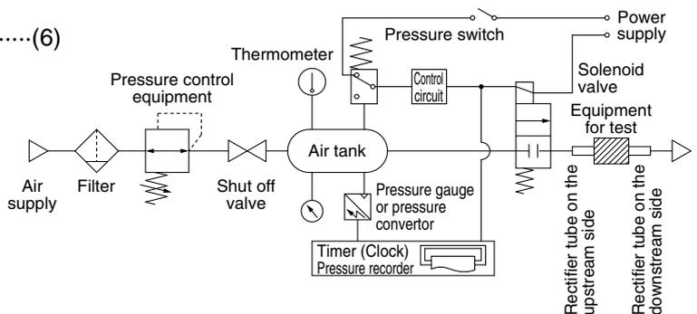
**Fig. (2) Test circuit based on JIS B 8390**
