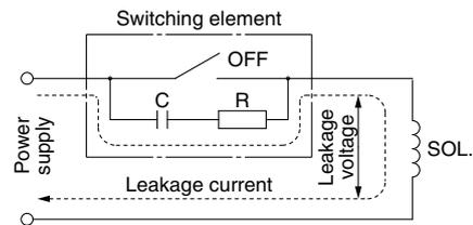
AC/Class B built-in full-wave rectifier coil: 10% or less of rated voltage
